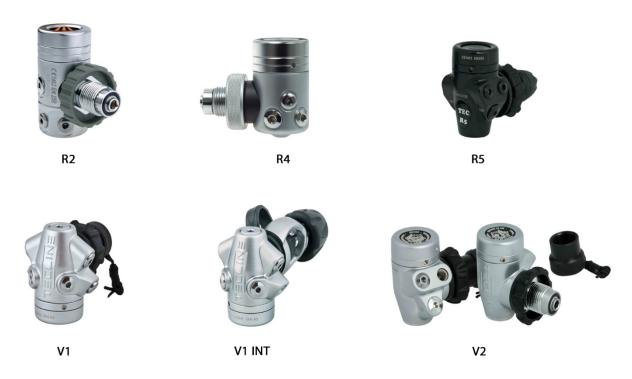
The second pressure reduction stages of Scubatech demand regulators are based on a standard, concurrent relief pressure reducing system. They are equipped with a Venturi nozzle with a setpoint adjusted by a diver that allows delivery of maximum flow of breathing gases. Using an adjustable deflector that directs appropriately the
